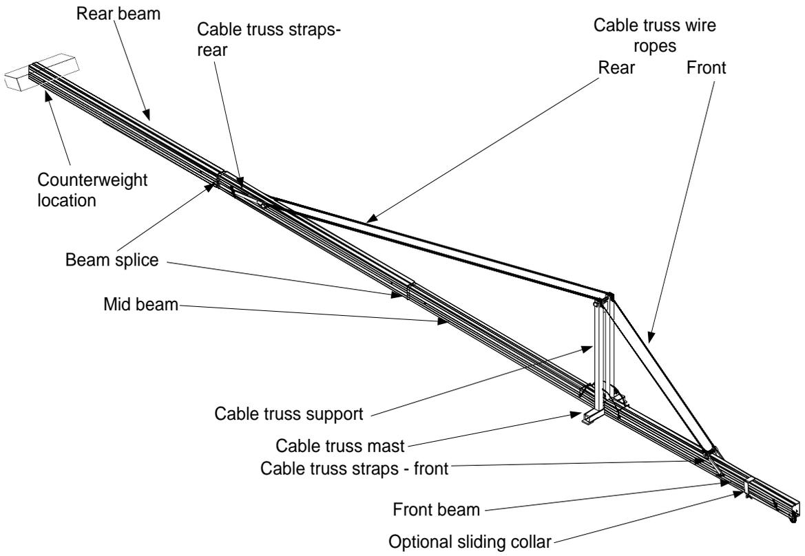
**Figure 11. Cable Truss System - 8' Reach**
