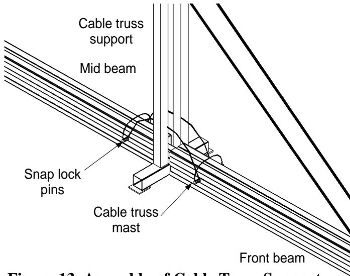
**Figure 13. Assembly of Cable Truss Support with Beams**
