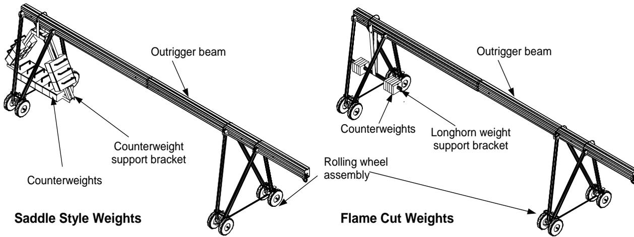
Figure 24. Rolling Outrigger
