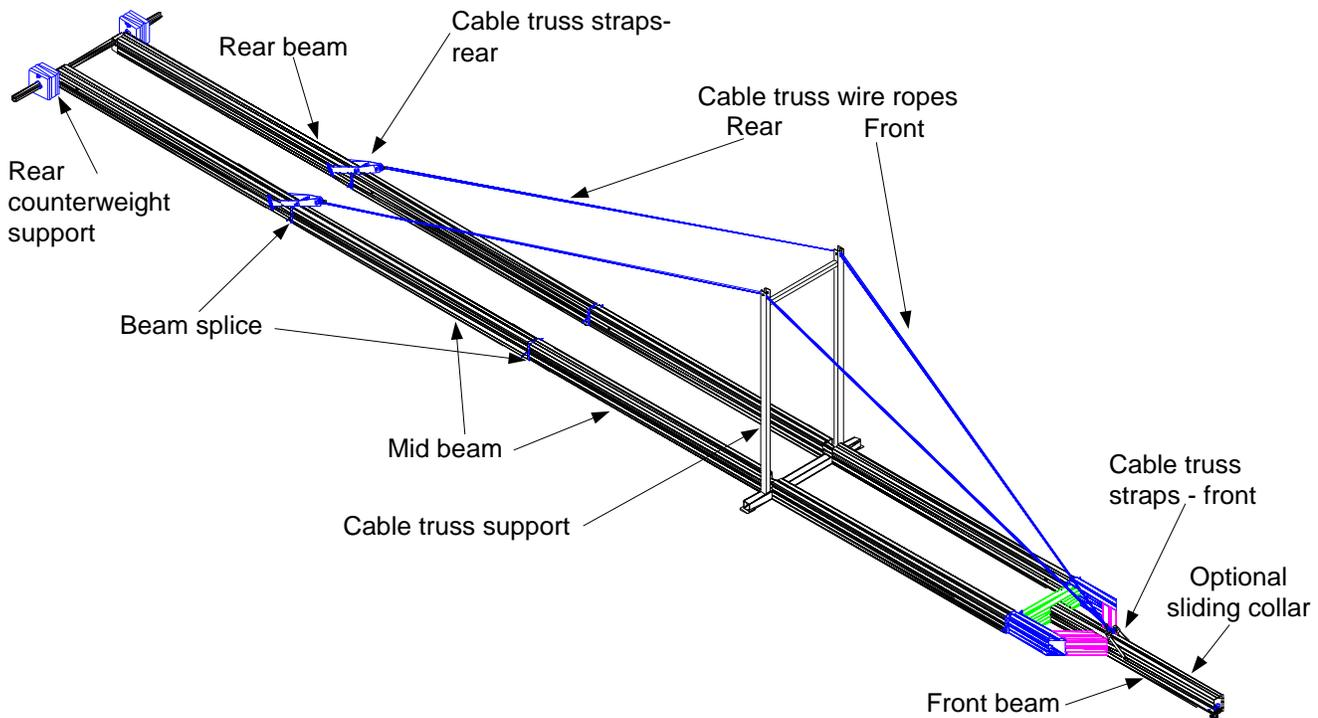
7. When moving the Cable Truss System into position ensure that the support for the front of the beam is located directly beneath the support feet of the Cable Truss Support. Do not support the Cable Truss System on either side of the Cable Truss Support as this places the load on the aluminum beam and not on the Cable Truss Support and can damage the aluminum beam.
