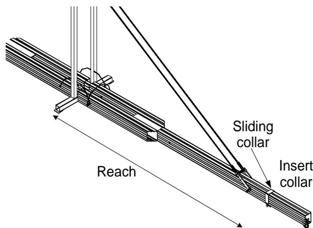
**Figure 17. Front Beam - Inner Section - Cable Truss Support Assembly**
