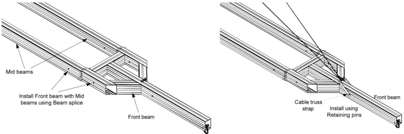
5. Pin the Cable Truss Strap (SP 166) to the Front Beam at a hole located approximately 3 feet from the front of the beam using a Retaining Pin (SP 169). Pin the Cable Truss Strap (SP 457) to the Rear Beam (both the beams) as shown using Retaining Pin (SP 169).
